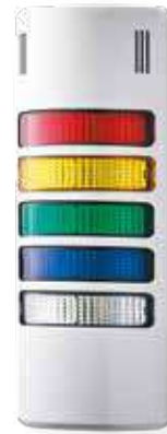
Order number: HD90-Q1036 Colours: red/yellow/green/blue/clear Function: LED steady beacon, buzzer steady or pulsing tone Housing colour: grey Nominal voltage: 24 V AC/DC
