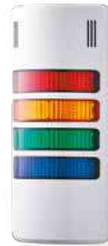
Order number: HD90-Q35 Colours: red/orange/green/blue/clear Function: LED steady beacon, buzzer steady or pulsing tone Housing colour: grey Nominal voltage: 24 V AC/DC
