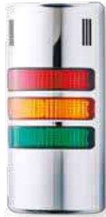
Order number: HD90-Q41 Colours: red/orange/green Function: LED steady beacon, buzzer steady or pulsing tone Housing colour: chrome Nominal voltage: 24 V AC/DC
