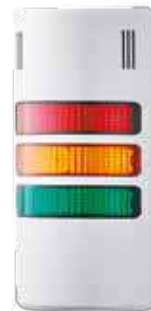
Order number: HD90-Q31 Colours: red/orange/green Function: LED steady beacon, buzzer steady or pulsing tone Housing colour: grey Nominal voltage: 24 V AC/DC
