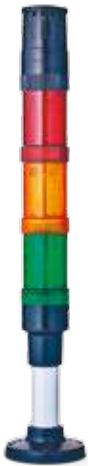
Order number: ECO40-Q31 Colours: red/orange/green Function: LED steady beacon, buzzer steady or pulsing tone Nominal voltage: 24 V AC/DC Type of mounting: Tube mounting (100 mm tube length)
