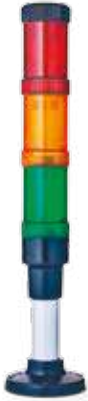
Order number: ECO40-Q01 Colours: red/orange/green Function: LED steady beacon Nominal voltage: 24 V AC/DC Type of mounting: Tube mounting (100 mm tube length)
