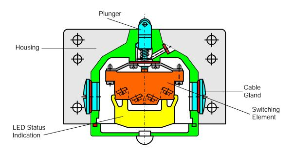
The system drawing shows in clear detail, the perfected design features of the TEKNIC EUCHNER precision limit switch. The material used by TEKNIC EUCHNER for the enclosure is a special aluminium alloy. The enclosure surface and thus the plunger guide are transformed by, a special surface coating into an aluminium oxide layer. This surface, combined with the hardened & polished plunger, offers particularly high wear and corrosion resistance.
